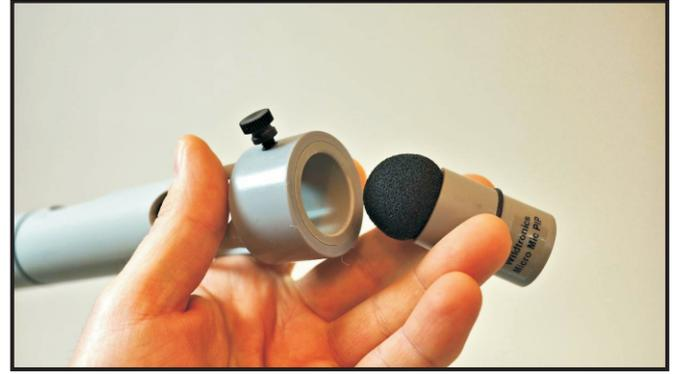
Step 2. Insert the Micro Mic PIP into the Mic Tube, wind screen first, until the O-ring is seated against the Mic Tube.
