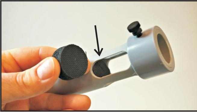
Step 1. Insert one of the foam cable clamps inside the Mic Tube as shown. This prevents resonance from the tube from affecting the microphone.
