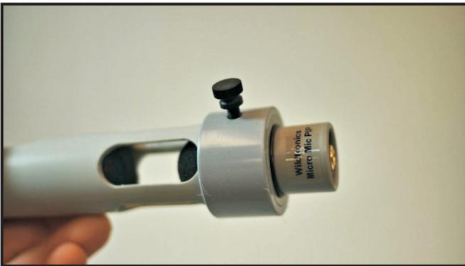
Step 3. Clamp the Micro Mic PIP in place by tightening the nylon thumbscrew.
