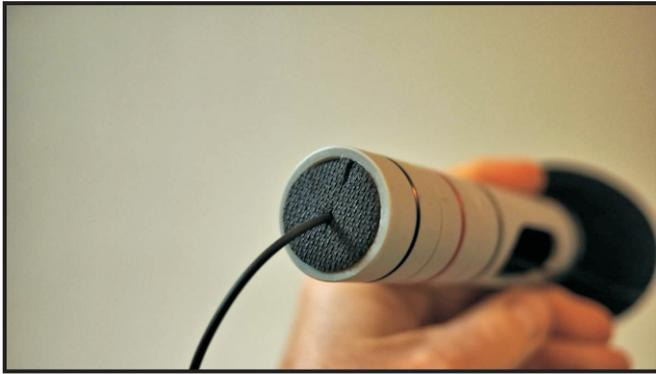
Step 7. Wrap the second Foam Cable Clamp around the 3.5mm cable and insert into the Mic Tube end. This secures the cable.
