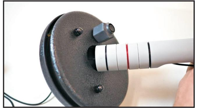
Step 8. Install the Mic Tube into the Front Plate and Back Plate that you have assembled to the parabolic dish.
