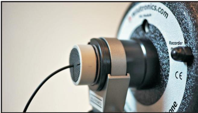
Step 9. Insert the Mic Tube so that the first black ring of the focus gauge is flush with the back of the clamp hub, as shown. Your mic is now at the focal point of the parabolic dish. Tighten the handle clamp.
