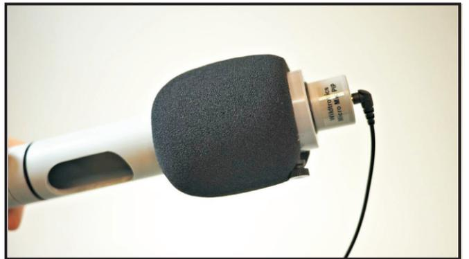
Step 4. Slide on the Windscreen, starting from the end opposite the Micro Mic PIP, until the large end touches the thumbscrew. Attach the 3.5mm cable.
