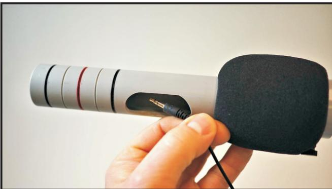
Step 5. Thread the 3.5mm cable through the cable slot of the Mic Tube.
